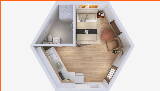
The HexPod: a modular, prefabricated unit that forms the building block of HexHomes' customizable housing system
